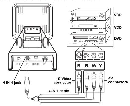
The cables are color-coded (black, red, white, yellow). Connect each colorcoded cable to the appropriate connector on your device.
